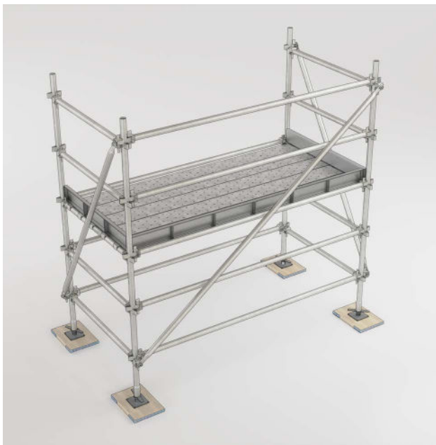
Figure 1: Example of a modular scaffold. Some scaffold components are omitted for clarity.
