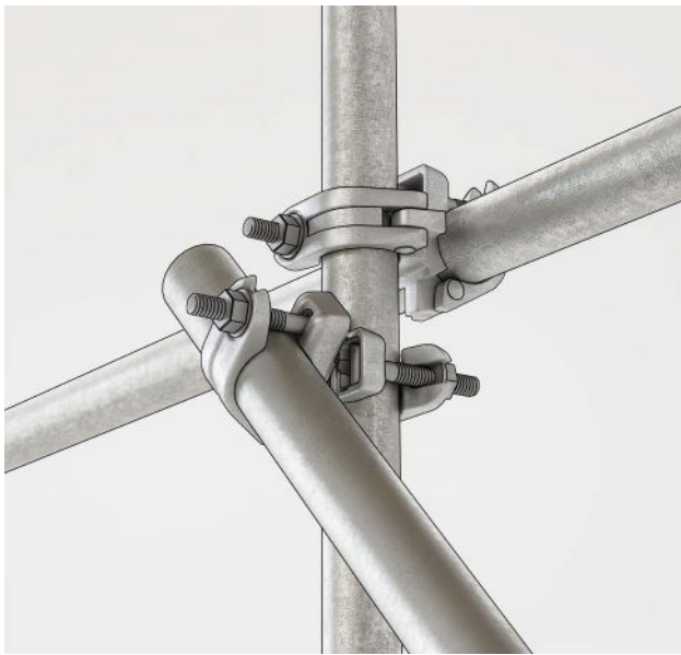
Figure 4: Example of a tube and coupler scaffold
