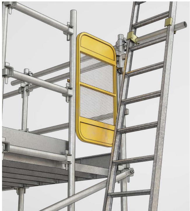
Figure 22: Use of external ladder access with self-closing safety gate
