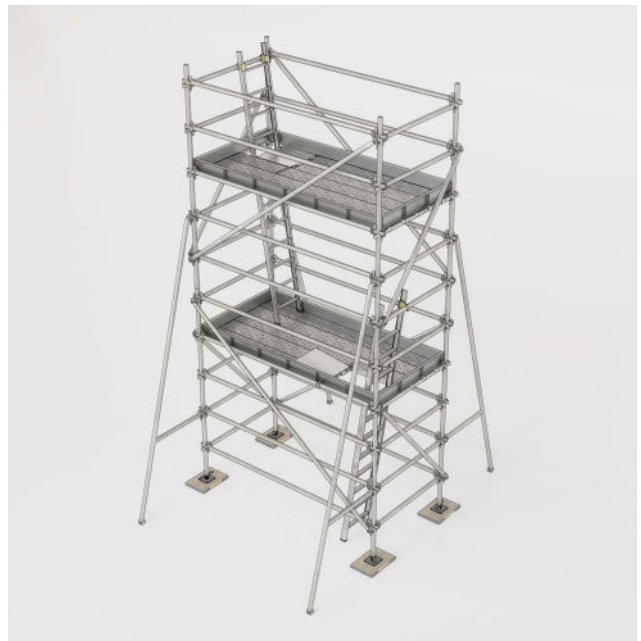
Figure 2: Example of a tower scaffold
