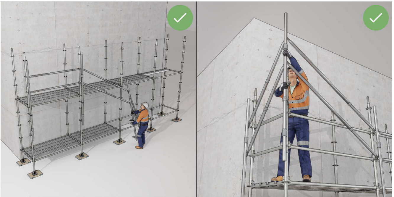
Figure 28: An example of scaffold erection method – advanced guardrail system. Some scaffold components such as toeboards are omitted for clarity.
