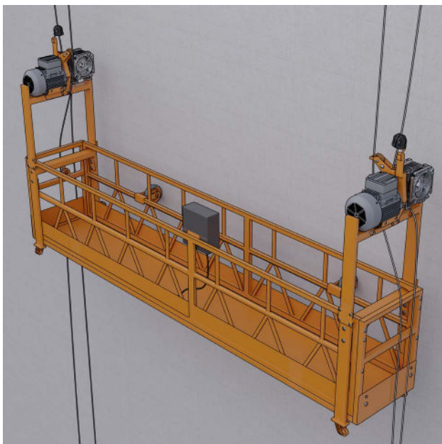
Figure 6: Example of a swing stage scaffold
