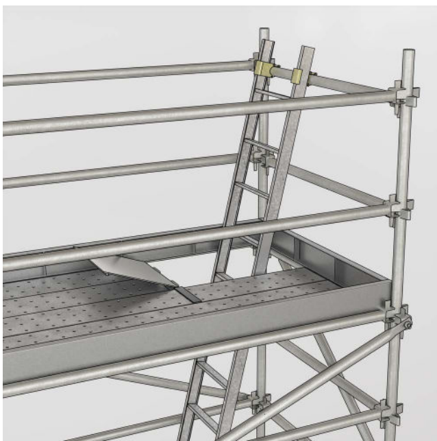
Figure 21: Use of internal ladder hatch
