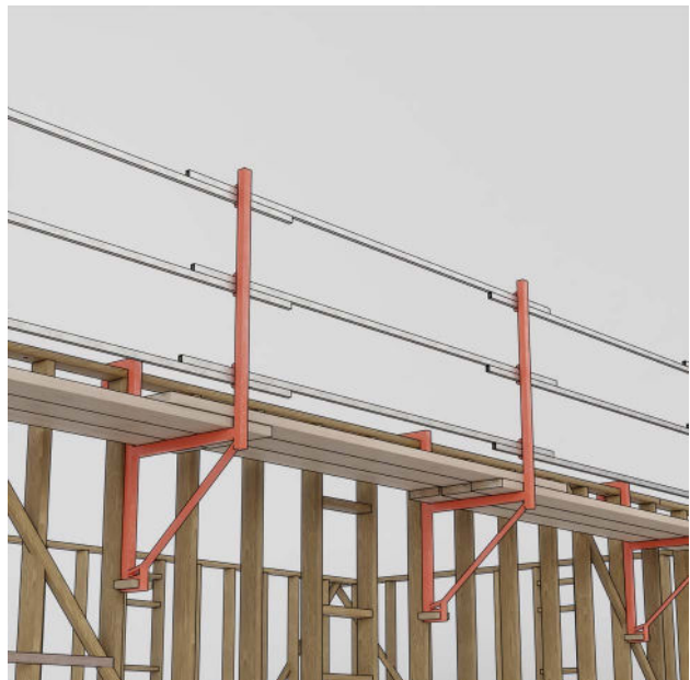
Figure 5: Example of a hanging bracket scaffold. Some scaffold components such as toeboards are omitted for clarity.
