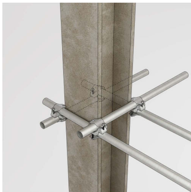
Figure 12: Box tie positively fixed around every side of a column or beam
